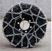
Apply the tensioning chain around the tyre and hook it on to an opposite piece of chain, while maintaining the tension on the tensioning chain by means of the tension spring. You are hereby allowed to shorten the tensioning chain yourself to a more acceptable length and subsequently re-attach the locking link and spring with the emergency or back-up links supplied separately.
