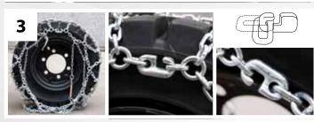
ATTENTION: the chain link is hooked into the special locking hooks crosswise. Thanks to the special locking hooks, it is impossible for the chain link to unhook lengthwise. It is possible to drive on a snowy surface if these locking hooks are situated on the tyre thread.
