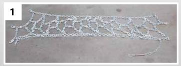
Lay the chain open on the ground as portrayed and make sure that links are not twisted or entangled. While doing this, check for any missing links or visible damage.
