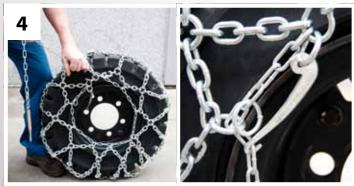
Now take the tensioning chain, tighten it firmly and lock it with the tightening lever. This can be done by using any free link.
