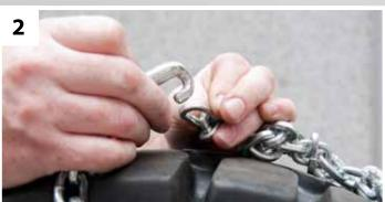
Place the tyre in the centre of the spread out chain. Fold the chain around the tyre and secure the locking hooks in the opposite loose link as shown on the picture.
