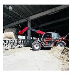
"There are some differences between telehandlers for construction and those for agriculture, such as a **difference in speed**. Since there are often many people working together on a site, safety is of the essence in construction and the maximum speed of equipment is limited to 20-25 km/h. In agriculture, fields are less crowded and the distance to the farm can be great, so speed is crucial. That is why farming equipment can often reach a speed of 40-45 km/h.
