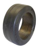
Press-on tyres should be replaced when **30% of the tyre's original tread rubber has worn away**. Using a tyre just 10% further than this will increase the **transmission of shocks and vibrations by 250%**. This exposes the forklift and the operator to damage and injury.
